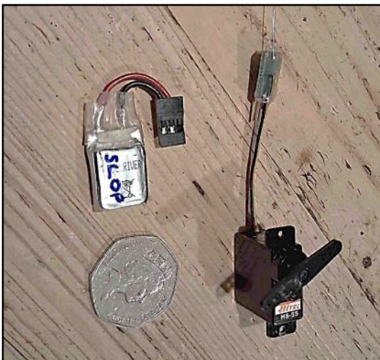
"Bodnar RDT receiver with battery and DT operating servo all of which has to be crammed into the fuselage"
