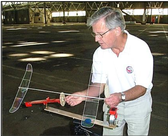
Bob Bailey transfers wound motor from winding jig to model and then sets his Ezebee on its way
